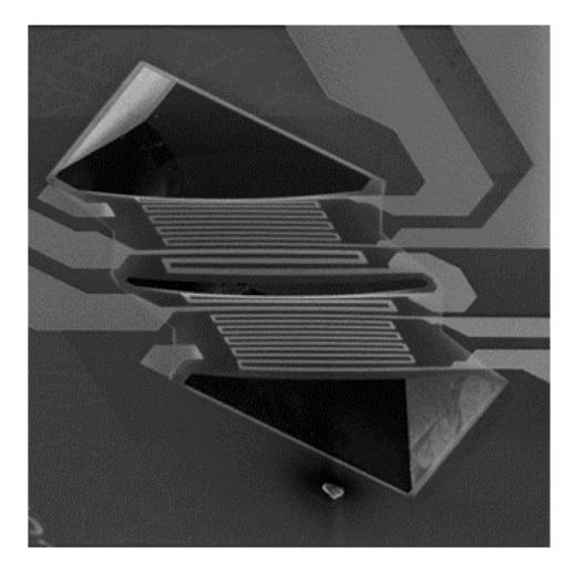
Magnification of the MEMS air flow, with the microheather, and temperature sensor. Overall chip size are ~ 1.7 x 3.3 mm.
